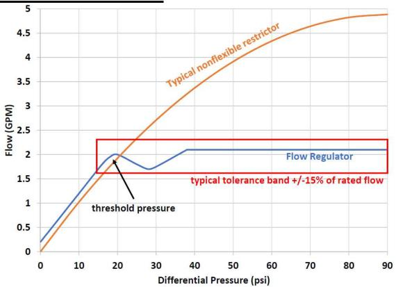
\*Typical flow curve of FR12 at 2 GPM.
