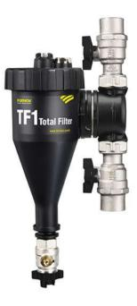
This award-winning TF1 Total Filter combines hydrocyclonic action with powerful Neodymium magnetic assemblies, to remove magnetic and non-magnetic contaminants from system water and contain them safely within the filter. It fits onto vertical and horizontal pipework, can be cleaned in minutes, does not restrict flow in any way.
