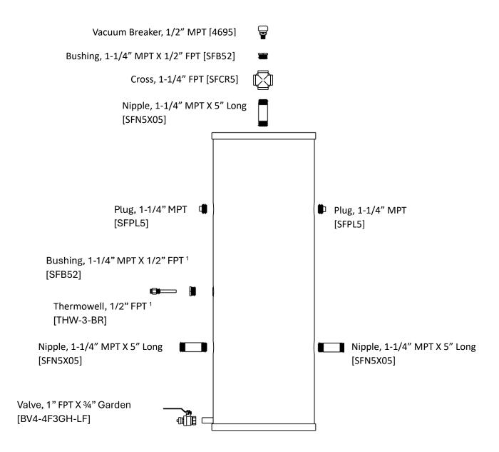
1. HCT-R2-\* 22 gallon buffer tank does not have a thermowell port.
