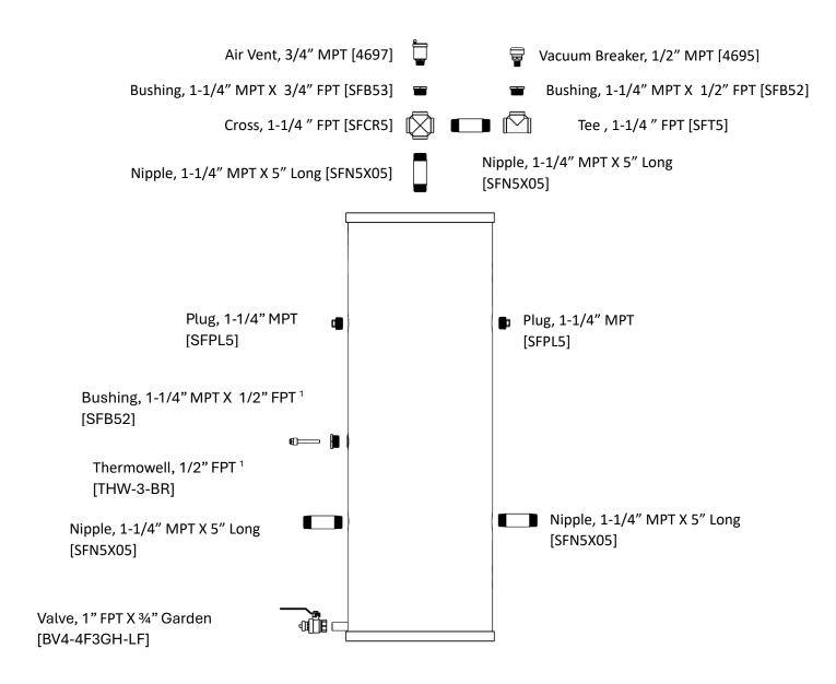
1. HCT-R2-\* 22 gallon buffer tank does not have a thermowell port.
