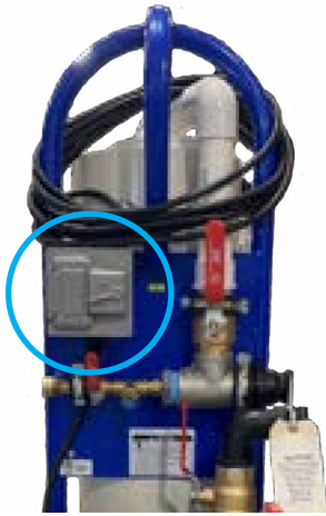
Figure 21: Remove electrical box from cart.
