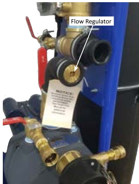
Figure 3: Flow regulator installed in 1-1/2" cam supply
