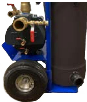
Figure 23: Disconnect the pump suction hose assembly. Shown removed
