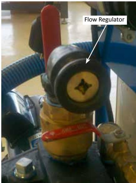
**Figure 3: Flow regulator installed in 1-1/2" cam supply**
