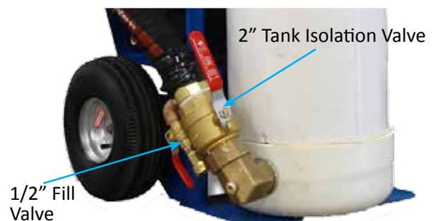
**Figure 5: Fill Valve/Tank Isolation Valve**
