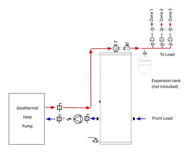
Note: Pressure relief valve not shown in above diagram (add to each diagram)
