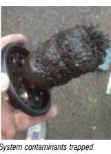
System contaminants trapped by the Fernox TF1 Total Filter
