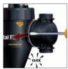
Pull the inlet/outlet port approximately 3mm away from the body to allow rotation to the required position.
