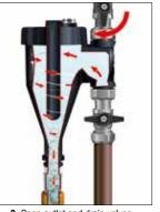
3. Open outlet and drain valves.
