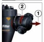
Push the inlet/outlet port back towards the body of the unit to prevent further rotation.
